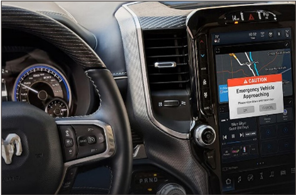
When responders activate apparatus emergency lights, approaching drivers receive real-time digital alerts to slow down and move over. These are delivered via apps, navigation systems, or mobile devices to drivers up to 30 seconds in advance and reduce the risk of collision by up to 90%.
